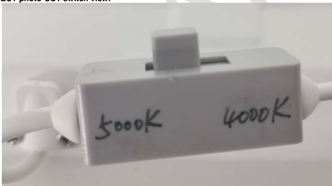
EUT photo-CCT switch view.
