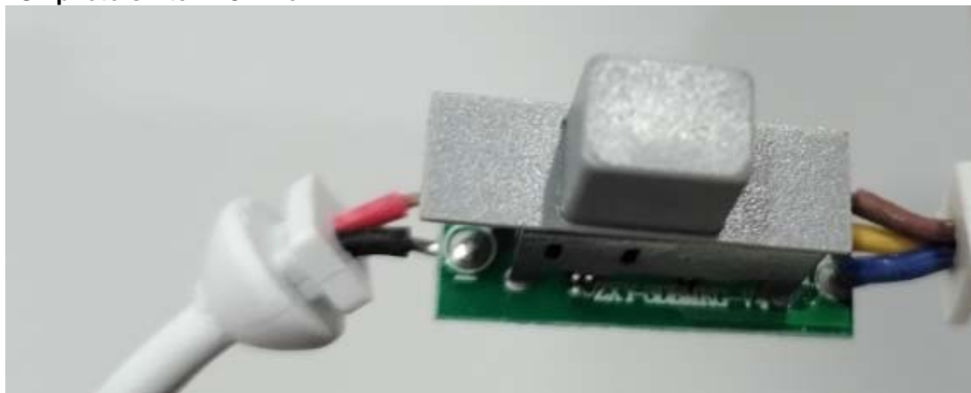
EUT photo-switch PCB view.
