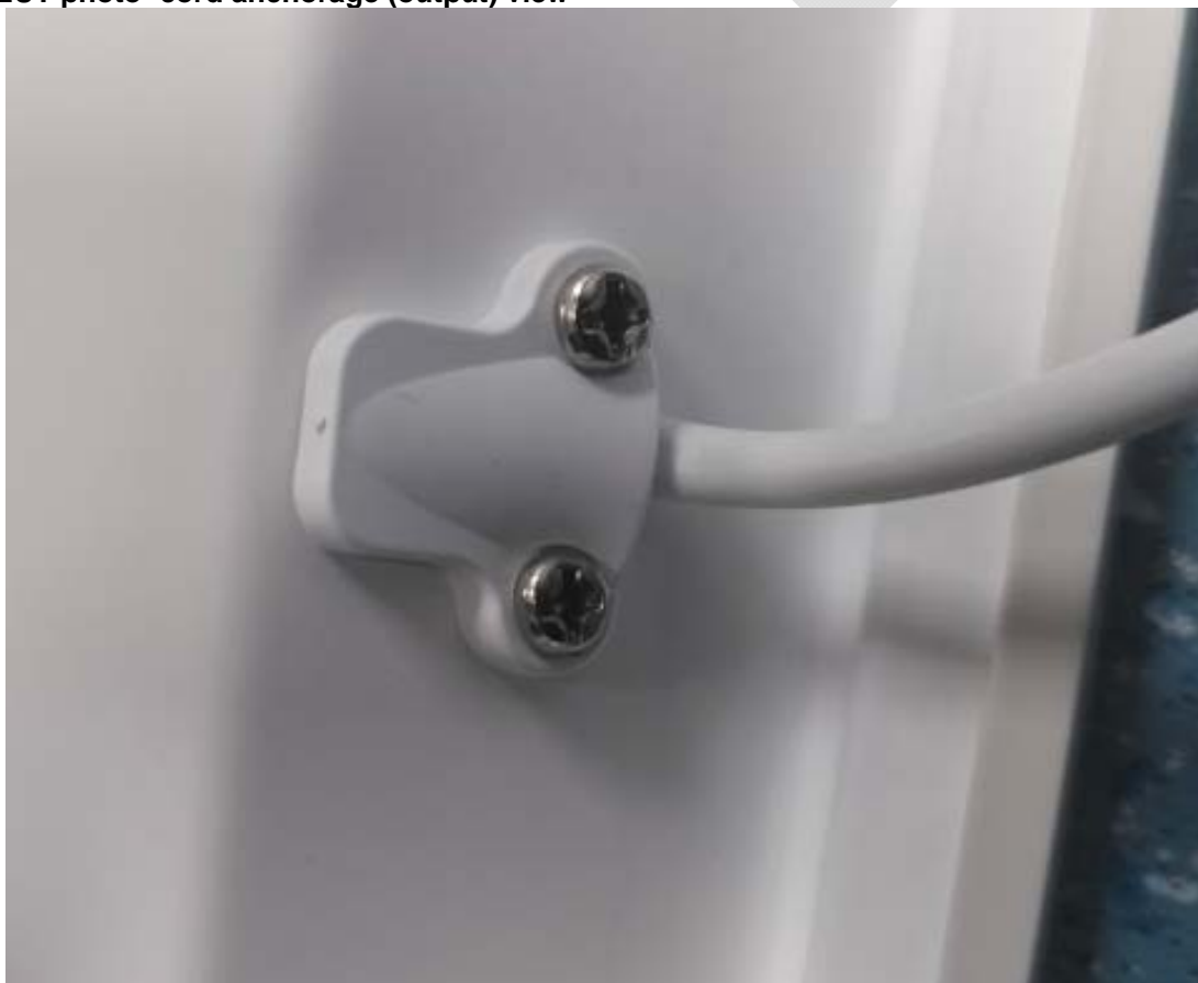
EUT photo- cord anchorage (output) view
