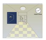
After last detection, the light will be dimmed down to the stand-by dimming level after holdtime.
