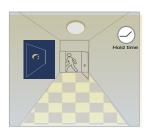
After last detection, the light will be dimmed down to the stand-by dimming level after holdtime.
