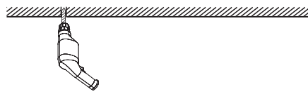
1. Drill a \varnothing 6\text{mm} hole
